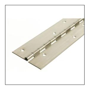
Heavy Duty Architectural Continuous Hinge Self Colour Stainless Steel – Staggered Holes 2000 x 102 x 2.5 x 7mm Pin – Stainless Steel 304/Grade 14 – Weight Load 160kg
